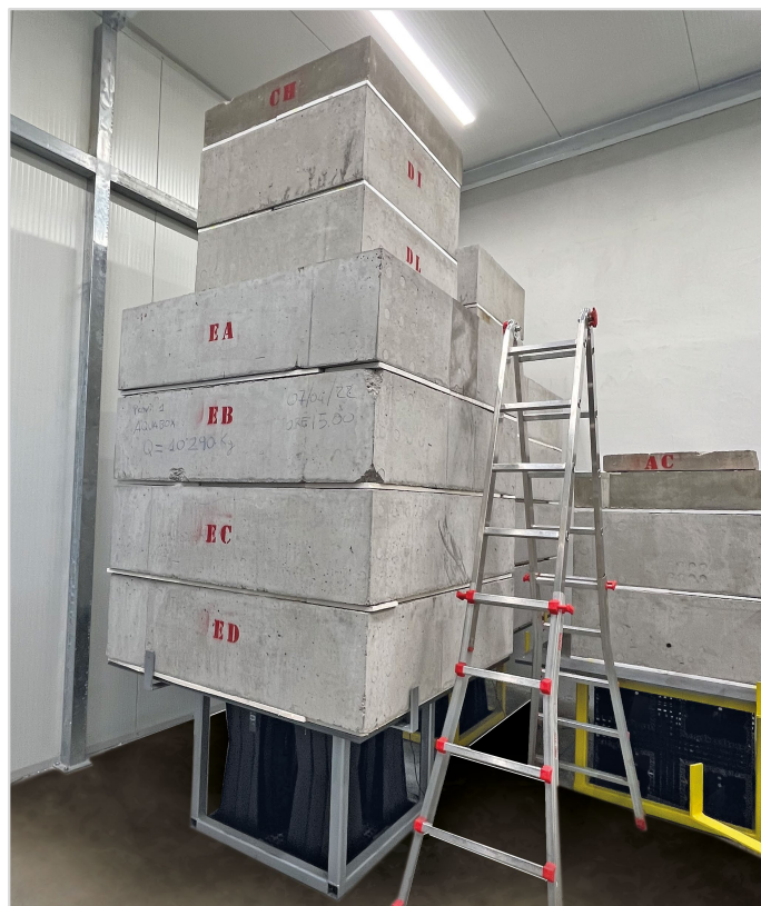
Aquabox load test concrete specimens
