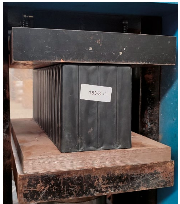
Strength test of the new polypropylene element
