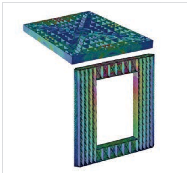
FEM analysis of the behavior of the elements and assembly under operating loads.
